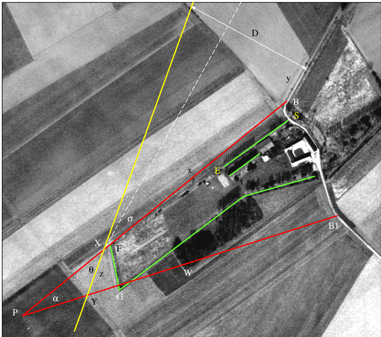
Figure 16: Aerial picture of 1995 with the critical lines of sight at B and B1, a fraction of the trajectory (in yellow) and the rows of high poplars that were present in December 1989 (in green).
