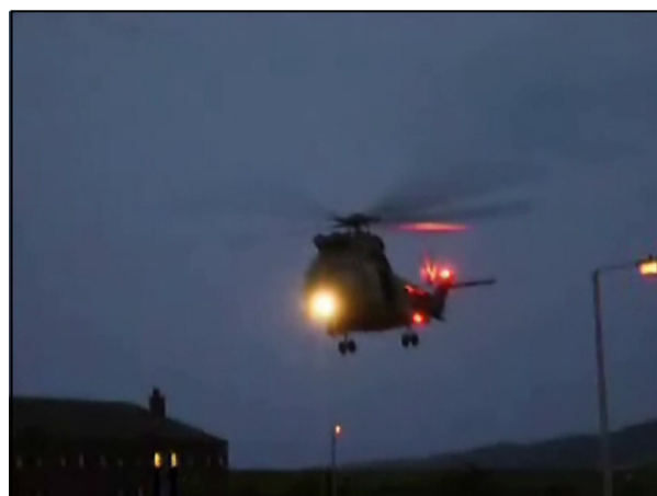
Figure 22: Landing lights of a SAE-330 Puma.
