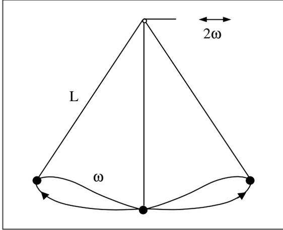
Figure 3: A pendulum can be a parametric amplifier
